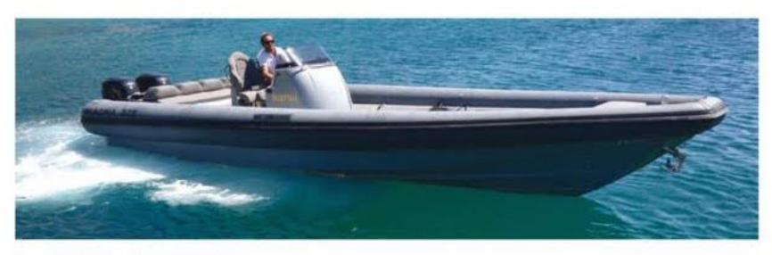
Length: 11 m - Beam 3, 25 m Engines: 2x300 hp SUZUKI
